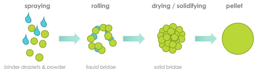
Also during granulation larger agglomerates are made from smaller individual particles.
