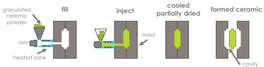
Cellulose ethers used for injection molding must be able to allow preparation of a thermoplastic mass which can be injected in the subsequent molding process.
